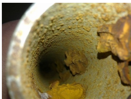
FIG. 4. REPRESENTATIVE EXAMPLES OF THE DEPOSITS PRESENT IN THE INTERIOR OF EXAMINED PIPES: A) REGION I PIPE, B) REGION II PIPE
