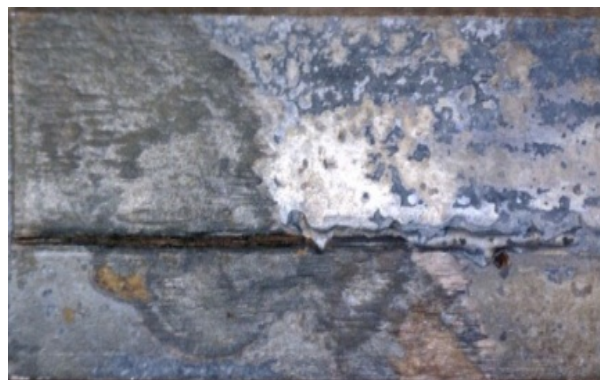
FIG. 5. REPRESENTATIVE EXAMPLES OF THE DEPOSITS PRESENT IN THE INTERIOR OF EXAMINED PIPES: A) REGION I PIPE, B) REGION II PIPE
